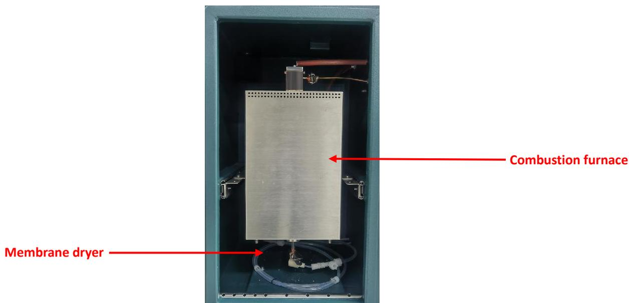
The combustion furnace is installed on the slide rail of the combustion chamber. During transportation or operation of the analyzer, the slide rail should be fixed inside the combustion chamber. When installing or replacing the reaction tube, remove the screws on the slide rail fixing plate, and the combustion furnace can be pulled out from
