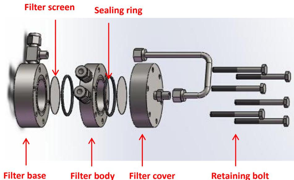
The filter screen should be cleaned or replaced periodically according to the cleanliness of the sample, and the wear degree of the sealing ring should be checked. Replace with a new sealing ring if necessary. We provide some filter screen and sealing ring for replacement. Please see Appendix A for details.
