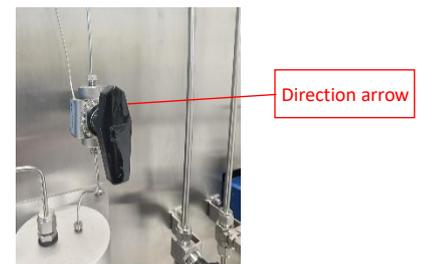
**Note: The direction indicated by the arrow of the manual valve1 is the analysis state of the sample or standard sample.**
