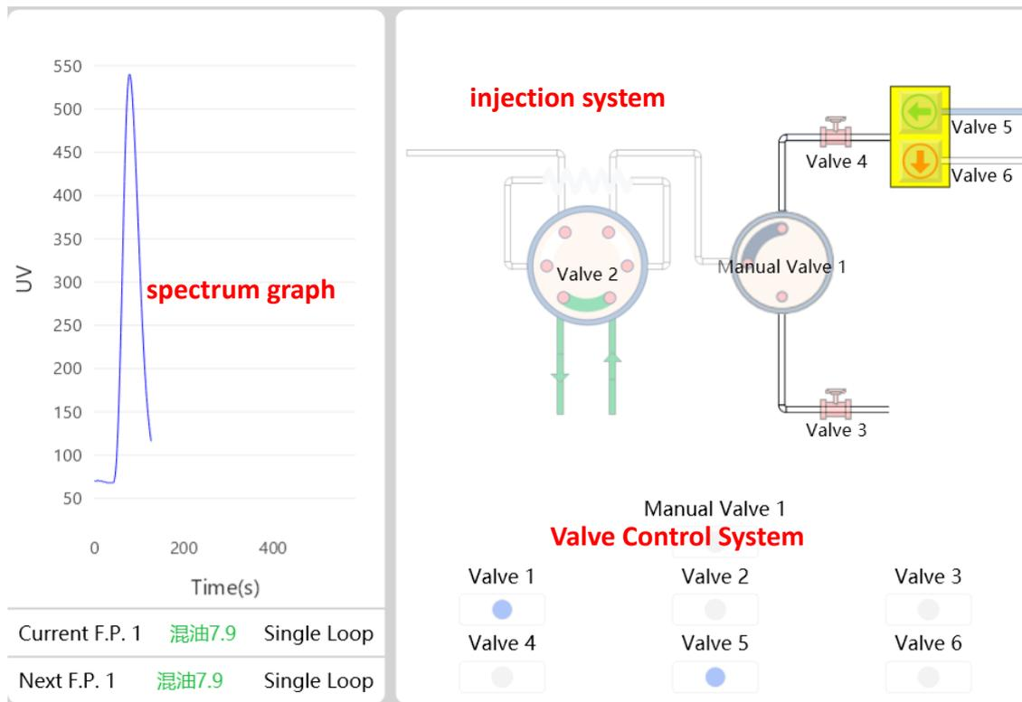
This page contains the real-time spectrum graph of the sample, the valve control system, and the sample injection system. You can also view the flow path samples being analyzed and the flow path samples to be analyzed soon through the current tasks and pending tasks.
