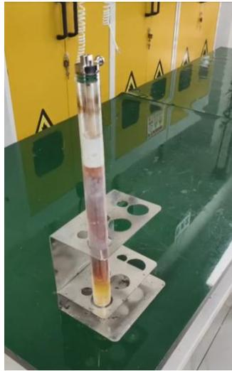
Note: When removing the pipe plug, you should be extremely careful. Pull the pipe plug vertically upwards to prevent breaking the sampling needle tube.
